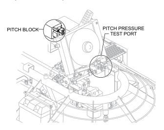
Figure 50. Pitch Block Location
